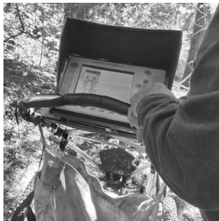
GPS Screen displaying underground electromagnetic disturbances.
