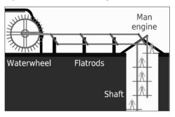
Another innovation in mining was the man engine. A man engine is a mechanism of reciprocating ladders and stationary platforms installed in mines to assist the miners' journeys to and from the working levels. It was invented in Germany in the 19th century and was a prominent feature of tin and copper mines in Cornwall until the beginning of the twentieth century.
